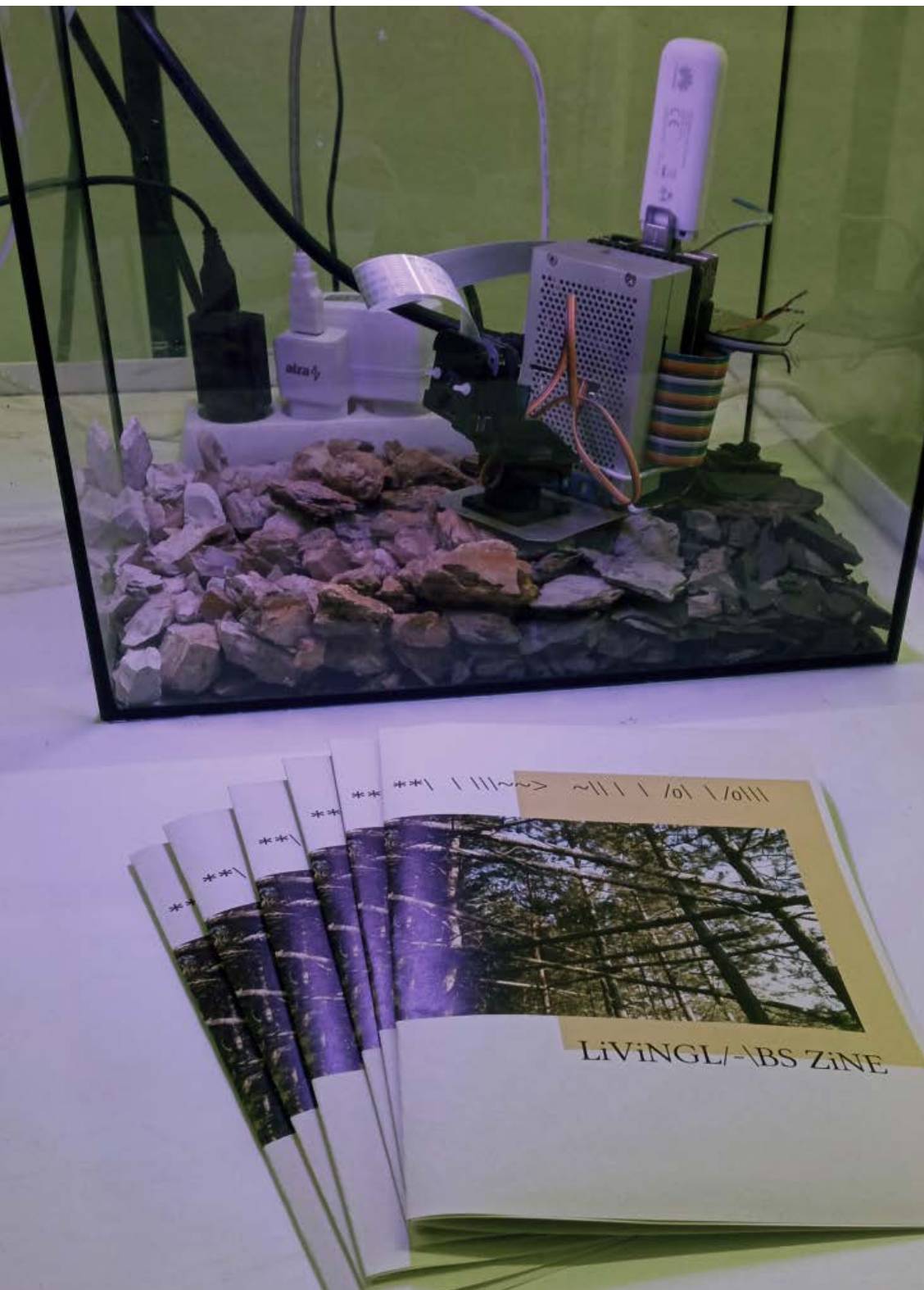
Figure 3: Klodner, M. et al. (2020-). Leaf node9 . Retrieved from https://webs.node9.org/channel/leaf . Solar-power designed field server for forest livinglab exhibited with Livinglabs zine in Entrance Gallery in Prague. Ecosystems and biodiversity are computationally supported with sensitivity to local resources, measured by environmental sensors. Leaf's open social network node and camera intermediate environmental art experiments from the field research or gallery space. Source: author
